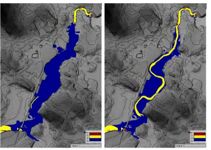
Figure 20. Existing (left) and Proposed (right) Channel Velocity During 2-Year Flow
